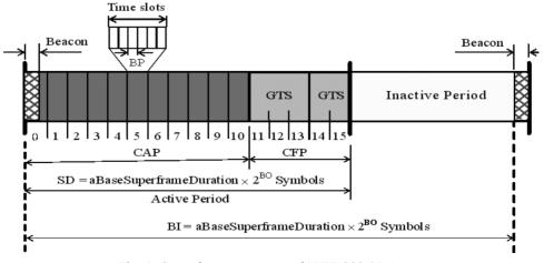
Fig. 1. Superframe structure of IEEE 802.15.4
