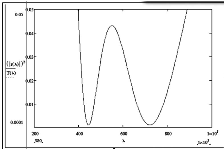
Figure 2.2. Graph of reflection coefficient of three-layer antireflection coatings  $\text{SiO}_2/\text{SiO}/\text{SiO}_2$
