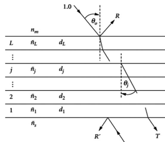
Figure 2.1. The L-layer thin films: from 1 ... j ... L, the index of each layer  $n_j$ , the real thickness for the layer  $d_j$
