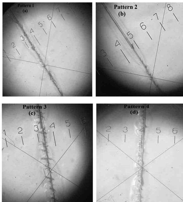
Figure 3.2. The incision shows the adhesion capacity of a three-layer film at different evaporation rates
