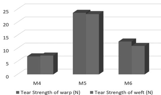
Fig 3. Tear Strength of warp and Tear Strength of weft of 3 materials for lining upper shoes
