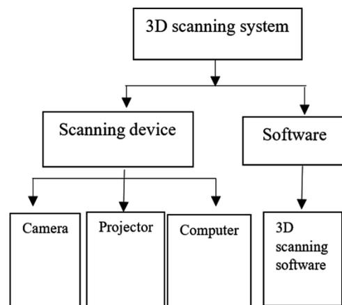
Figure 3. Structural diagram of 3D scanning system
