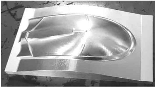
Figure 15. Mould core of computer mouse case
