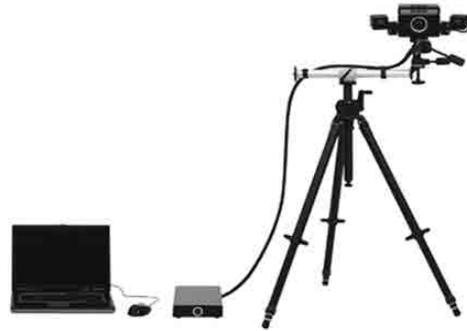
Figure 2. ATOS scanner system
