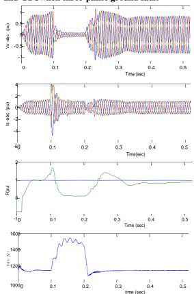
**3.2.** The proposed control strategy for the RSC and GSC when three-phase ground fault
