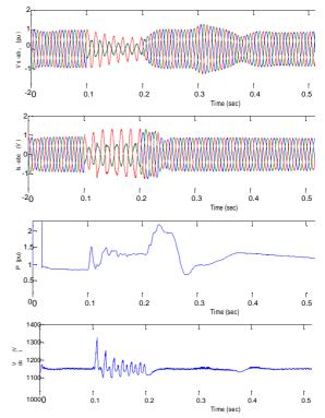
Figure 9. Vs, Is, Ps, Vdewith the proposed control strategy for the RSC and GSC when the phase A and phase B to ground fault
