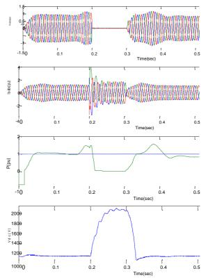
Figure 7. Vs, Is, Ps, Vdc with the traditional vector control strategy for the RSC & GSC Figure 7 showed that the waveforms of Vs,
