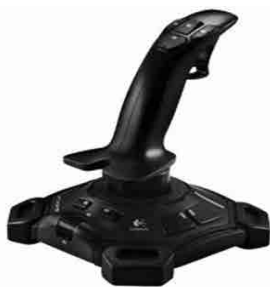
Figure 6. Joystick Attack 3 issues commands via USB
